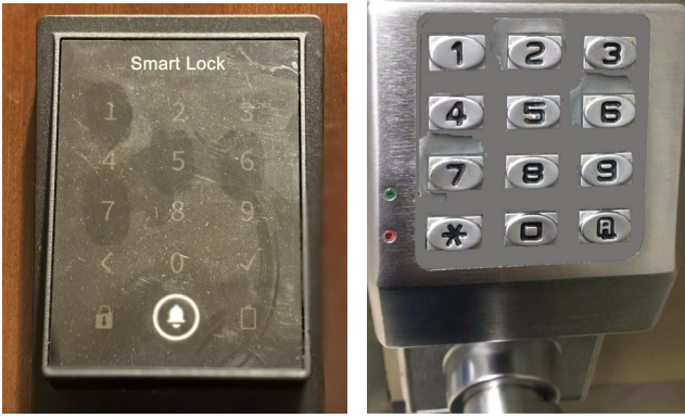
Fig. 1. Access control keypads that leave/leak input traces in the real world. We can clearly see that the left user’s password consists of the four digits 1, 5, 6, and 7, while the right user’s password contains 2, 6, and 7. Using this side-channel information, the attacker can perform mask password guessing to significantly increase her guessing success rate (see Fig. 5).
